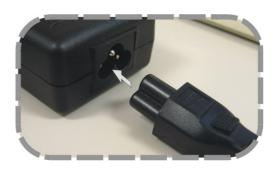
2. Connect the connector end to the device and the plug to an outlet.
