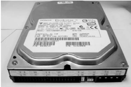
3) Connect IDE cable and 4-pin power adapter cable on your hard drive.
